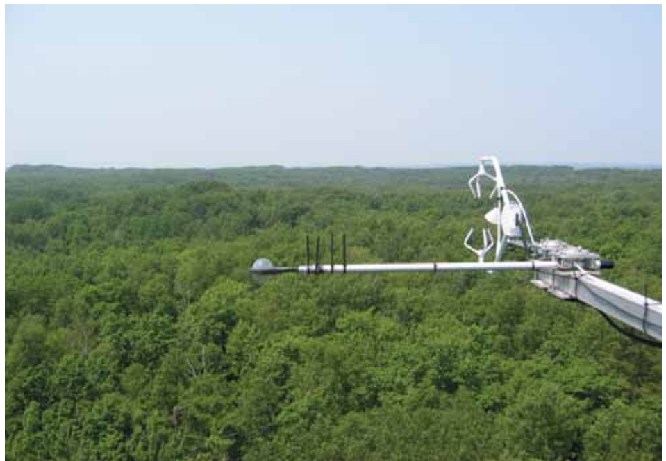
Sensors on 150-foot towers above the forest canopy measure the flow of carbon dioxide into and out of the trees at the University of Michigan Biological Station. In Great Lakes forests, carbon flow during photosynthesis and soil respiration results in the net storage of about 0.7 tons of carbon per acre each year.
